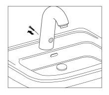
Block the sensor for 2 seconds.
